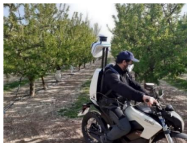
Fig. 2. Photograph of the terrestrial LIDAR scanning the almond trees.
